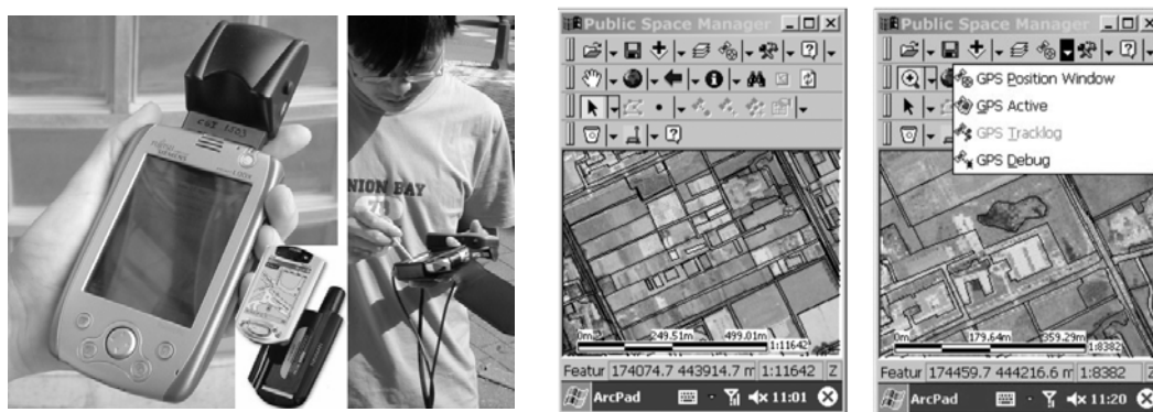
Figure 3: A PDA/GPS/ArcPad application to do field work
